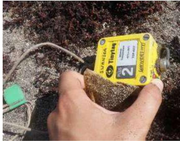
**Figure 17 Temperature data logger**
